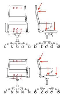
DURABILITY TESTS OF THE ARMREST Application point compared to the most forward point of the armrest: 100mm Load: 400 N Number of cycles: 60.000
