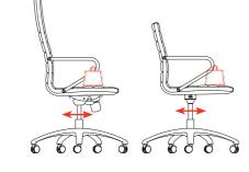
VERTICAL STATIC LOAD AT THE CENTRE OF THE ARM Load: 900 N - 750 N
