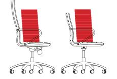
RESISTANCE TO ROLLING OF THE SEAT WITH NO LOAD Test speed: 50 mm/s Measured resistance: 27 N Mininum allowed resistance: : 12 N
