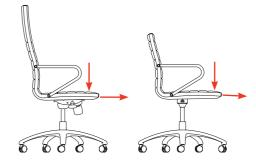
STATIC LOAD ON THE FRONT OF THE SEAT Load: 1.600 N Number of cycles: 10
